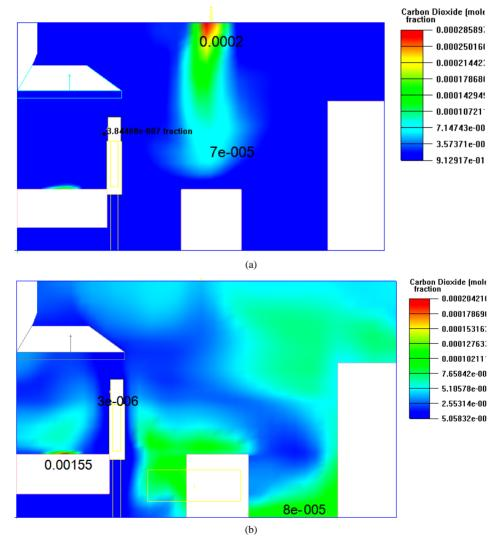
Figure 7. X = 2.9 cut plane  $CO_2$  distribution. (a) For MV system; (b) For DV system.
