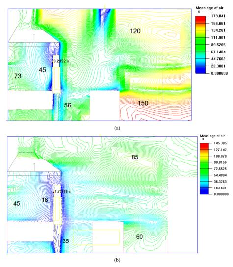
Figure 8. X = 2.9 cut plane mean age of air distribution. (a) For MV system; (b) For DV system.
