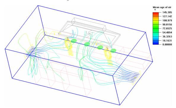
Figure 3. Airflow track for DV.
