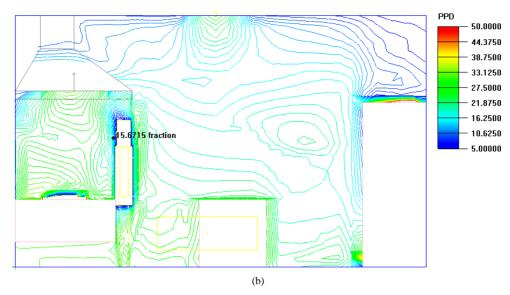
Figure 6. X = 2.9 cut plane PPD distribution. (a) For MV system; (b) For DV system.
