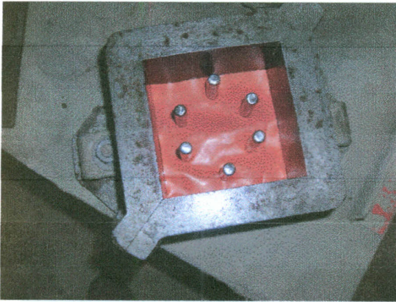
Plate 3.2: PVC block with Polythene sheet lining in the Mortar Cube
