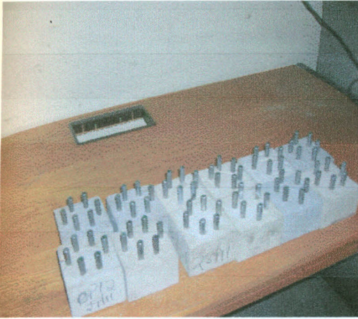
Plate 3.3: Mortar Cubes Simulating Reinforced Concrete
