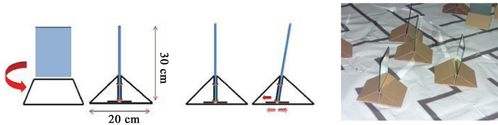
Figure 8. Mirrors and sensor's base, their rotations.
